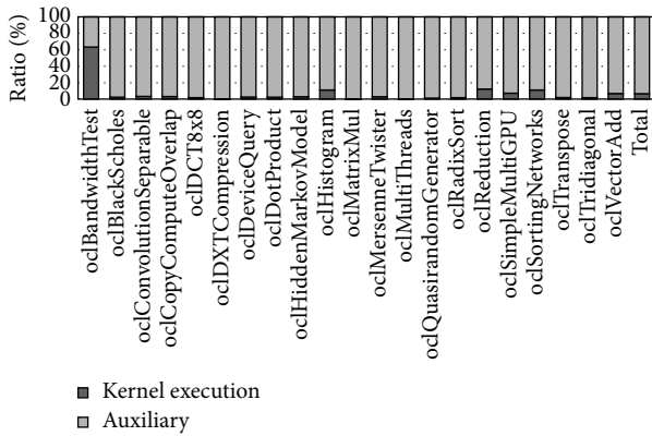
FIGURE 3: Execution time distribution of kernel execution and auxiliary API functions.
